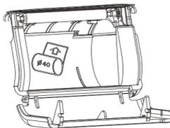
Install the paper roll as shown, with the paper coming from the top, and pull out 6 inches of paper.
