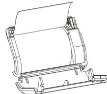
Close the paper hatch and tear off excess paper at a 45-degree angle.
